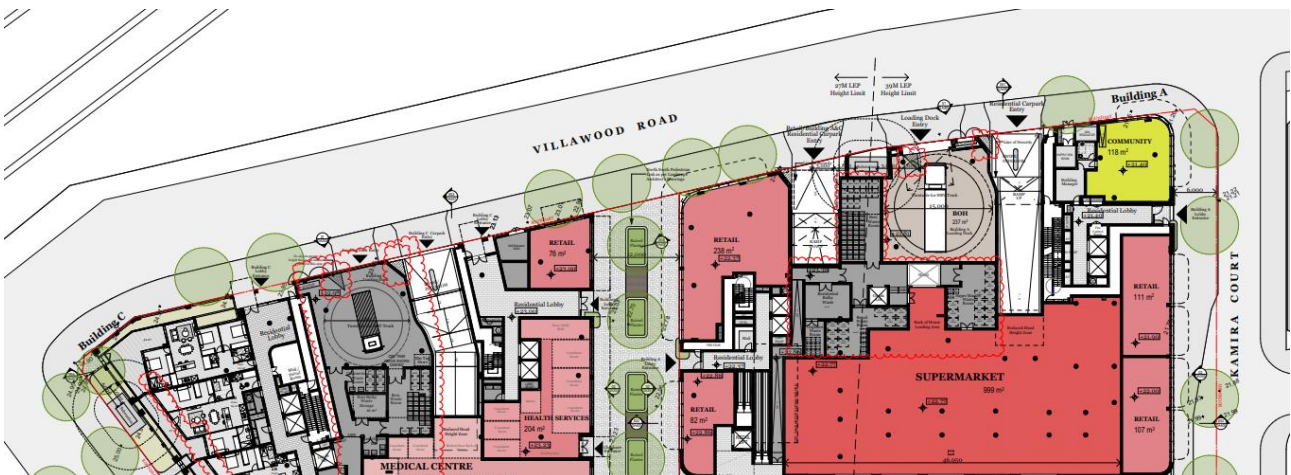
Location of three (3) vehicle crossings and two (2) loading bays along the Villawood frontage.
